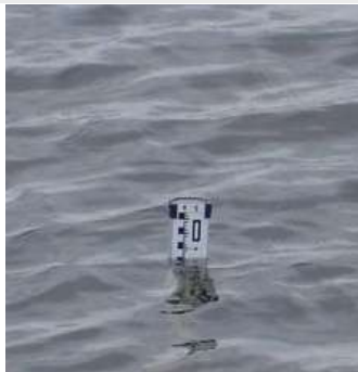
Water layer thickness
